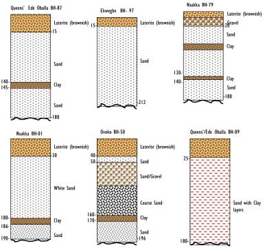
Figure 8: Some other Lithologic logs of boreholes around the study area (Modified after Egboka, 1983) NOTE: Depths are in metres
