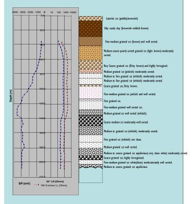
Figure 5: Log and lithological results of the borehole (E04), at the Energy Centre, University of Nigeria, Nsukka.
