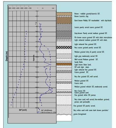
Figure 6: Log and lithological results of the borehole (Z05) at Zenith Bank, Nsukka Town.
