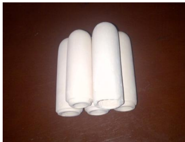
Fig. 4. Water filter candles that have been fired
