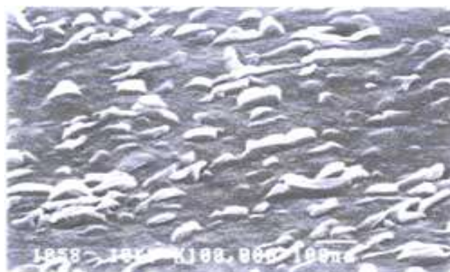
Figure 1: Nanomer particles protruding from a plasma-etched polymer matrix. Source: Nanocor
