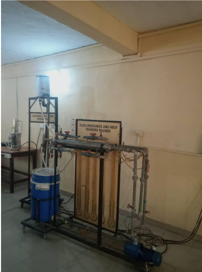
Figure 6: Isometric view of combined Fluid Mechanics and Heat Transfer Trainer, plus its auxiliary Constant Head Water Circulator.
