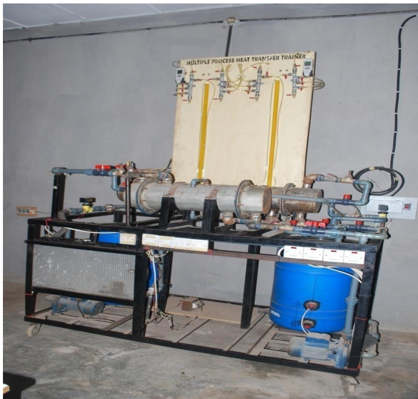
FigureC-4: The photograph of front view of prototype multiple process heat transfer trainer after full installations of pumps and measuring instruments
