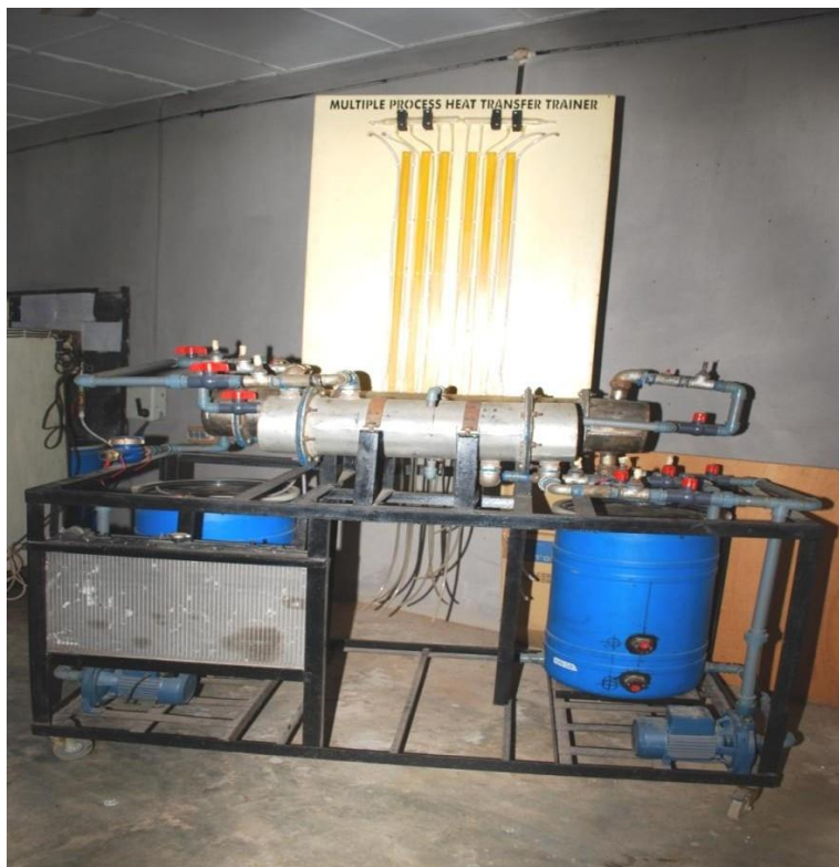
Figure C-2: The photograph of front view of the prototype multiple process heat transfer trainer before installation of measuring instruments' manifolds
