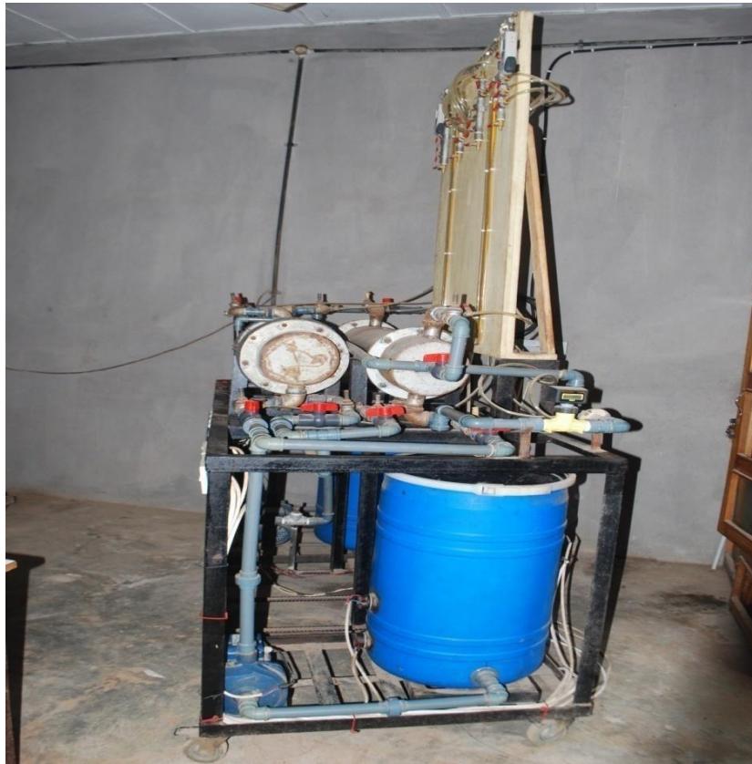
Figure C-5: The photograph of side view of prototype multiple process heat transfer trainer after full installations of pumps and measuring instruments
