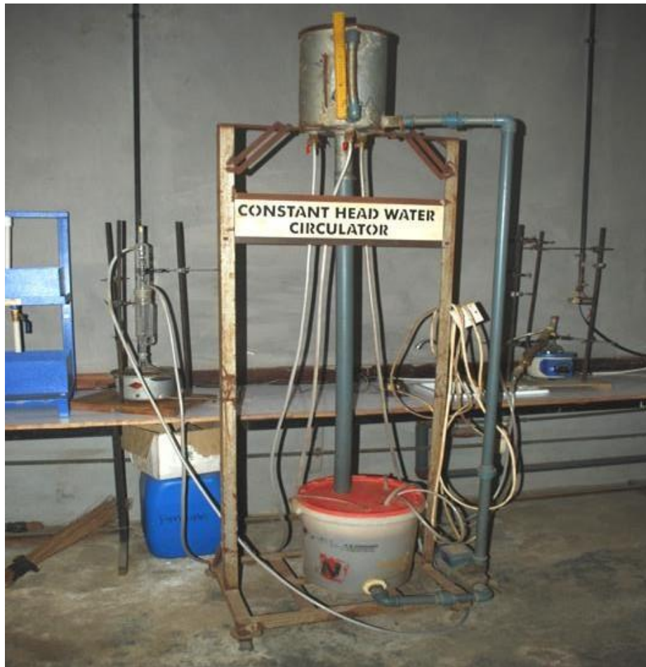
FigureE-1: The photo graph of the prototype constant head water circulator
