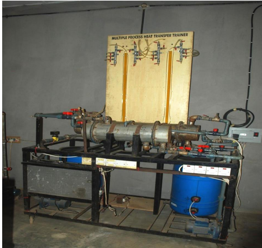
FigureC-3: The photograph of front view of prototype multiple process heat transfer trainer before installation of measuring instruments' manifolds
