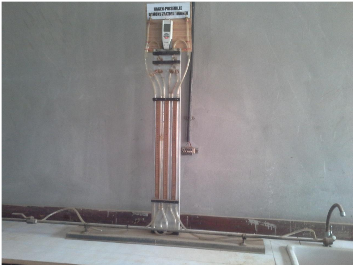
FigureM-1: The photograph of the prototype Hagen-Poiseuille demonstration trainer.
