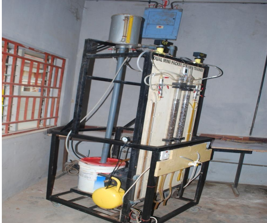
FigureD-3: The diagonal view photograph of the prototype minidual packed column trainer after fitting the electronic manometer
