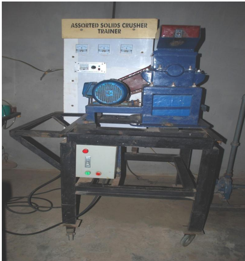
Figure K-1: The photograph of assorted solids crusher trainer after completion and commissioning
