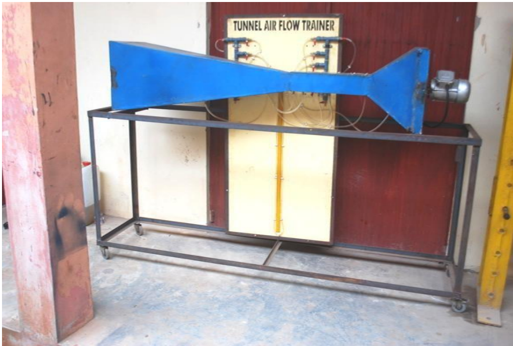
Figure L-1: The photograph of the prototype venturi air tunnel trainer after completion and commissioning
