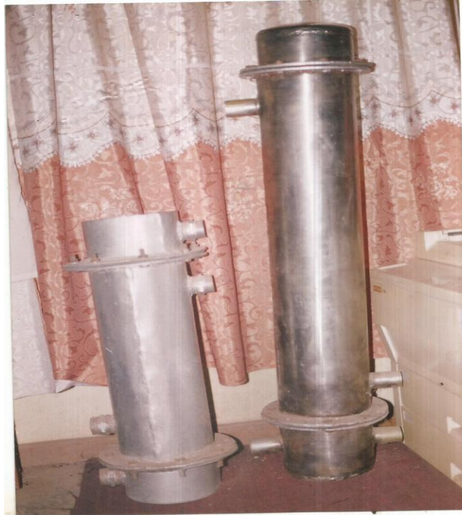
FigureC-1: The photograph of the 1-2 and 1-2 shell and tube heat exchangers before transformation into prototype multiple heat transfer trainer
