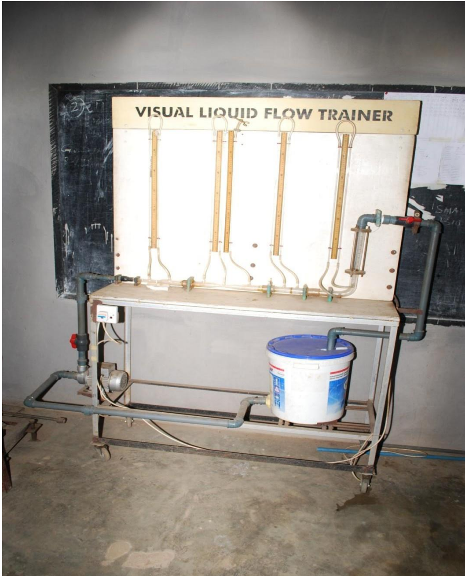
Figure I-1: The photograph of the prototype visual liquid flow lab trainer after completion and commissioning
