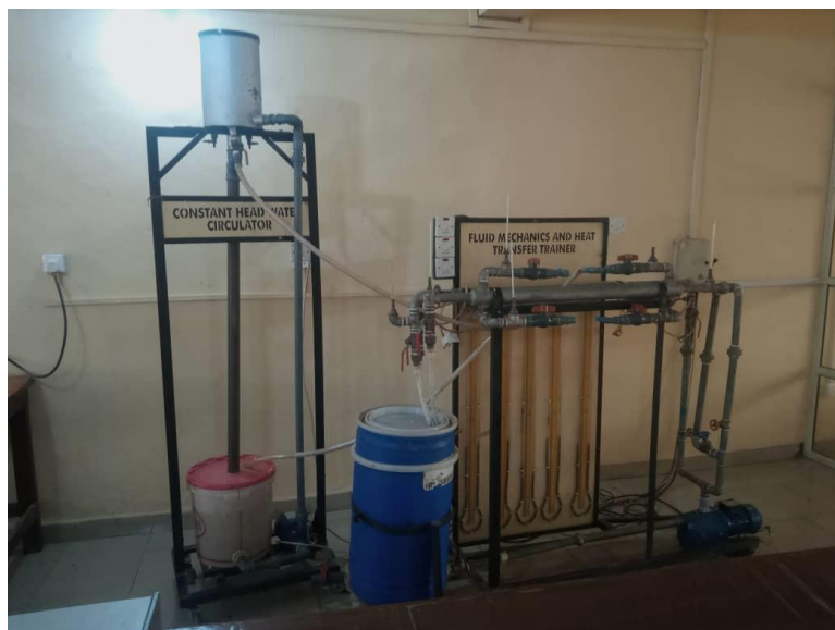
Figure 5: Front view of combined Fluid Mechanics and Heat Transfer Trainer, plus its ancillary Constant Head Water Circulator.
