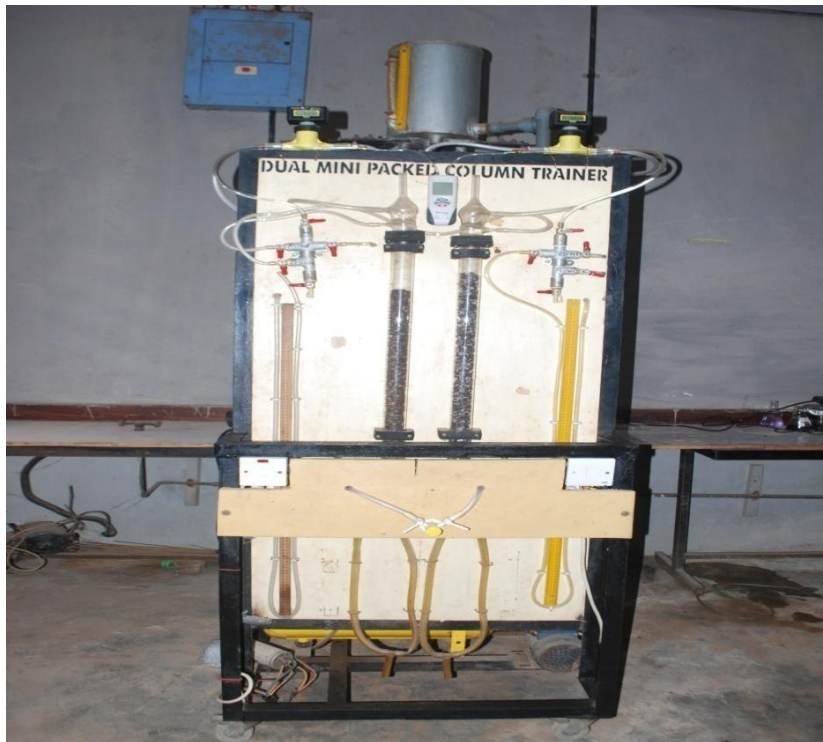
FigureD-2: The front view photograph of the prototype minidual packed column trainer after fitting the electronic manometer
