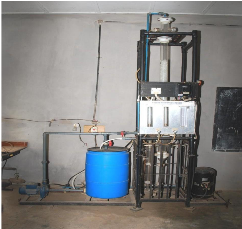
FigureG-1b: The photograph of the prototype pilot plant packed absorption tower before renovation and upgrade.
