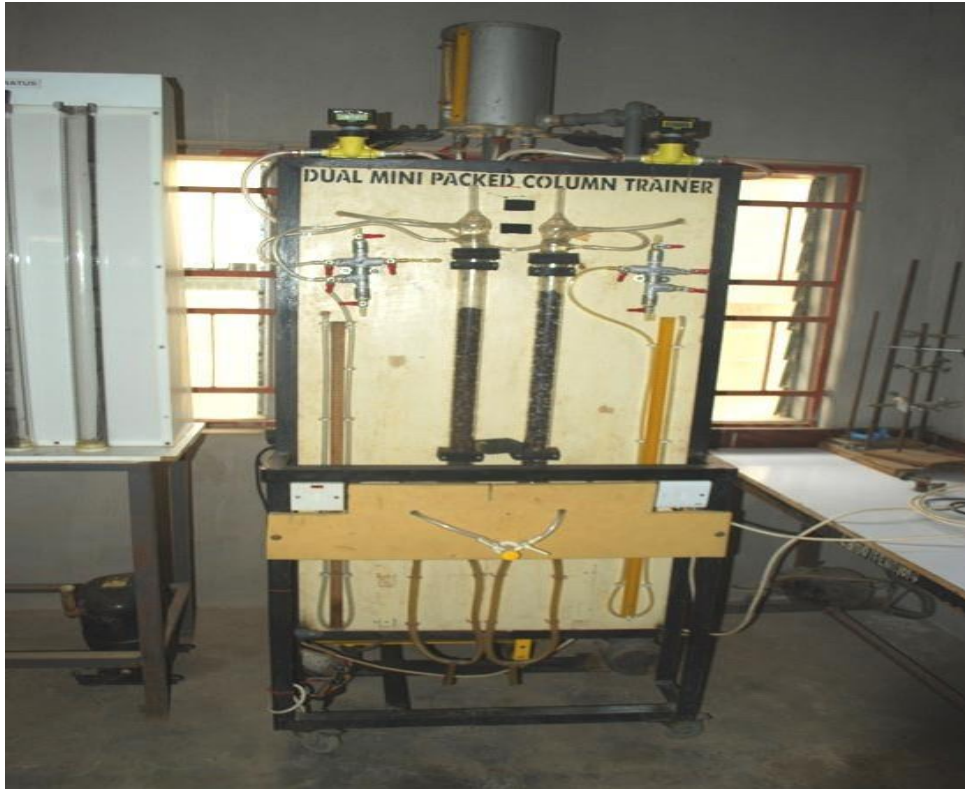
Figure D-1: The front view photograph of the prototype mini dual packed column trainer before fitting the electronic manometer
